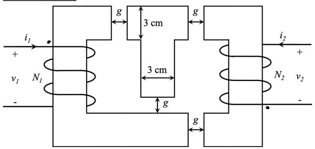
Two coils are wrapped around an iron core with infinite permeability as shown. Coil 1 has 400 turns while coil 2 has 100 turns. The air gap g is 2.5 mm and the depth into the page is 2 cm. Neglect fringing.
