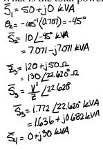
$\overline{S}_{tot} = \overline{S}_1 + \overline{S}_2 + \overline{S}_3 + \overline{S}_4$   $\overline{S}_{tot} = 58.706 + j.23.606 \text{ EVA}$ = 63.276 \( \frac{1}{2} \).908° \( \text{EVA} \)
