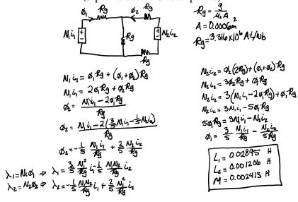
c) What is the RMS magnitude of the open circuit voltage on coil 2 if  $i_1(t)=10\cos(377t)$ ? (5 points)
