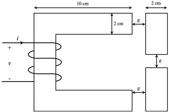
A coil is wound 250 times around an iron core with infinite permeability (dimensions given above) that has an air gap of 5 mm and a depth into the page of 3 cm. Fringing effects are included.
